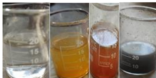
Figure 2. Stages of formation of nanoparticles with oil extract by changing colors.
